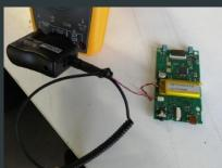
The adapter contains a battery used to power the device to be tested.
