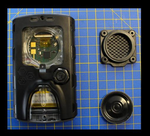
Remove D2-RC1-BOTTOM symmetrically from the D2-RC1-MAIN.
