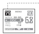
Note: Depending on the frequency setting used, a target's conductivity is perceived differently by the detector. The digital conductivity display may therefore vary depending on the frequency.
