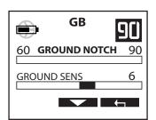
Adjust the machines ability to track soils according to their intensity. This makes it possible to avoid tracking on soils with a low mineralisation.
