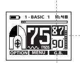
**Mineralisation strength**. The higher this value, the more mineralised the ground is. Pump the coil up and down several times to evaluate the mineralisation strength. If the level is low, there is less of a need to make any adjustments.
